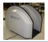
SSD integrates three orthogonal and complementary sensors: electromagnetic differential (EMD) metal detection for weapon detection, Quadrupole Resonance ED technology, and Trace Explosives Detection (based on the MobileTrace<sup>®</sup> engine)
